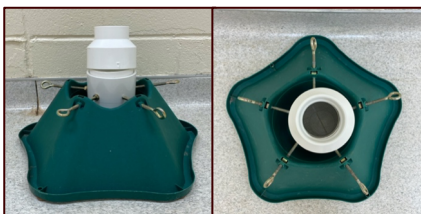
Figure 1: Sample presentation apparatus. Samples were placed in glass jars inside the PVC containers, supported by tree stands.
